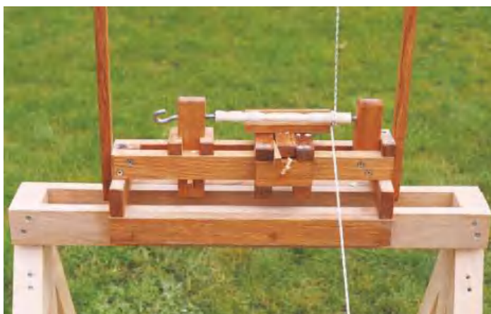
▲ Pic.2 Pieces up to about 50mm diameter can be turned on this size of lathe
